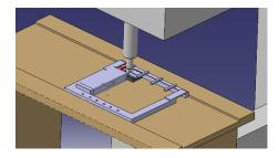
**Image 3:** During eClinching, a push-button-like joint is created in a cold forming process made of several sheet layers.
