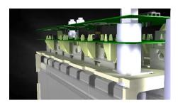
**Image 2:** The battery is divided into twelve modules for proper and particularly safe handling. The individual cells are connected in series using so-called busbars.
